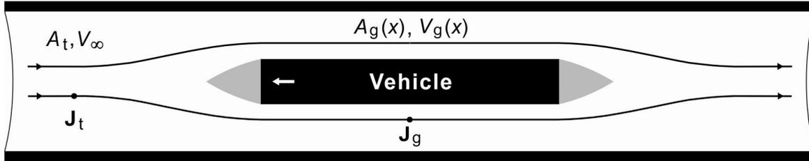
**Figure 3. Model of gap flow.** The vehicle is moving right-to-left in the hydrogen tube. Point  $J_t$  on a streamline is far ahead of the advancing vehicle and  $J_g$  is on the same streamline in the gap. Distance  $x$  describes the one-dimensional flow through the gap.
