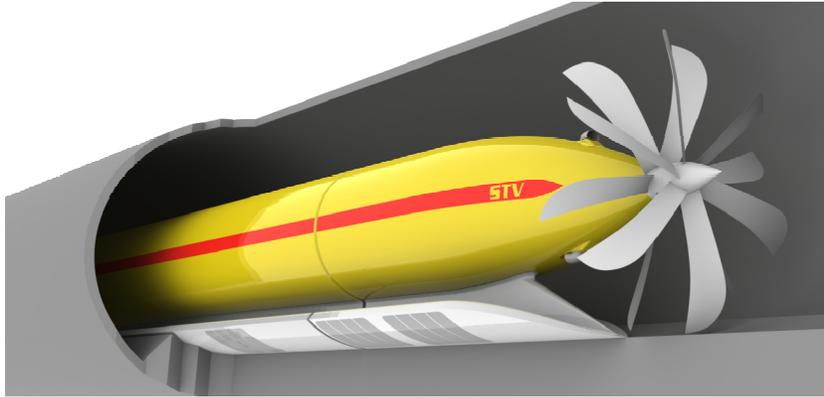
**Figure 1. Supersonic tube vehicle in its hydrogen tube.** Cutaway model shows front locomotive, first passenger car, contra-rotating propfan propulsion, and levitation on aerostatic gas bearings. Fuselage outer diameter is 2.69 m, propeller diameter is 4.5 m, and tube inside diameter is 6.4 m. Tube hydrogen pressure is slightly above outside air pressure.
