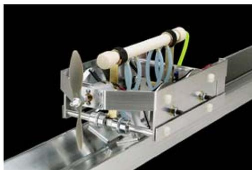
.....and the first small working model of the fuel cell tube train built and studied by Vehicle Projects.
