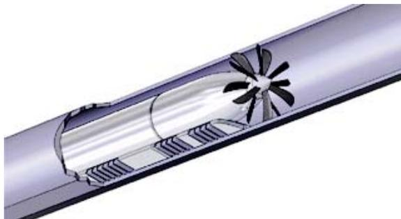
Riding the Tube: a conceptual visualization of the fuel cell-powered supersonic tunnel train being studied by Vehicle Projects.
