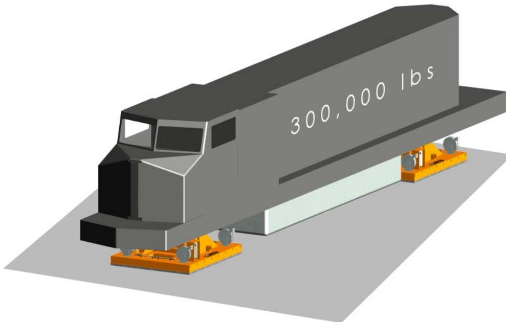
**Fig. 6. Commercial application of aerostatic air bearings.** Externally pressurized air bearings support this locomotive while it is moved across a factory floor during manufacture. The bearings use compliant gas seals. (Illustration, except for the underlying plane, courtesy of Airflow, LLC)
