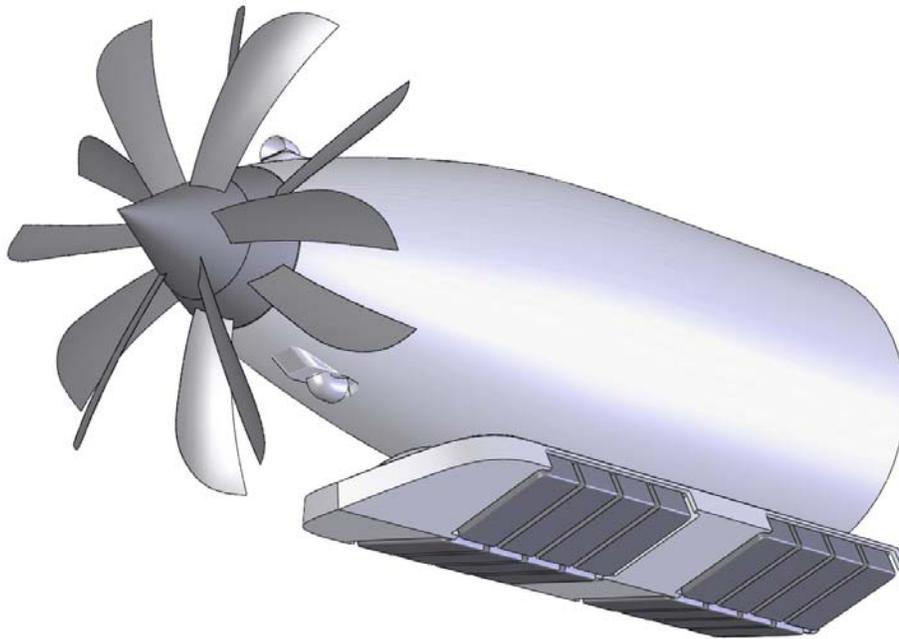
**Fig. 4. Detail of locomotive.** The model shows the contra-rotating propfan and four-segment gas-bearing pads. Each group of four segments, whose gas pressure and geometry can be independently and actively varied, constitutes a *bearing pad* and corresponds to a truck (bogie) of a conventional rail vehicle.
