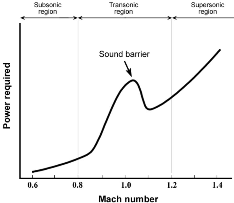
**Fig. 1. Aircraft power as a function of Mach number.** When the vehicle speed reaches the transonic region, Mach 0.8 – 1.2, propulsion power rapidly rises. The power peak located at Mach 1 is termed the “sound barrier.” (Adapted from references [1,2]).
