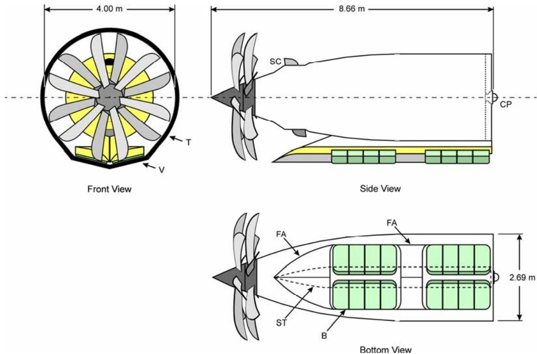
**Fig. 5. Scale drawing of locomotive in the hydrogen tube.** T = hydrogen tube, V = vee-way, SC = hydrogen scoop; CP = genderless ball-and-socket coupling, FA = fairing for streamlining the bearing-pad unit, ST = strut supporting fuselage above gas-bearing unit, B = four-segment gas-bearing pad conforming to vee-way.
