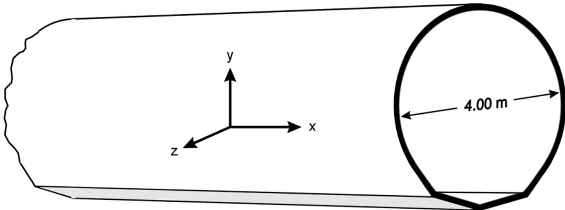
**Fig. 2. Schematic of the hydrogen tube.** The vee-way, the levitation and guidance rail, is shown at the bottom of the 4.00-m inside-diameter tube. The x-axis of the modified right-handed coordinate system is the center of the tube, which may curve in three-dimensional space. The y-axis is orthogonal to the x-axis and bisects the symmetrical vee-way. The z-axis is orthogonal to both x- and y-axes.
