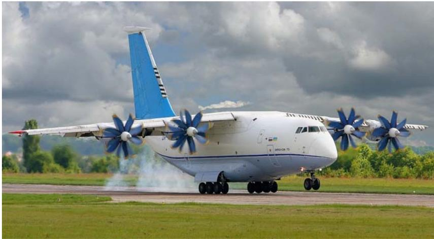
**Fig. 3. State-of-the-art Antonov propfan airplane:** Analysis of the maximum cruise speed of the propfan-driven STV is based on aerodynamic extrapolation of the cruise speed (Mach 0.74) of the 41 MW, 145 t Antonov An-70 (photo source: Oleg Belyakov).
